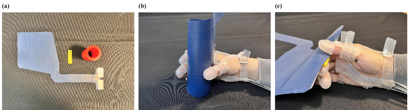
Figure. S12 Experiment setup using a pressure pad. (a) Measurement devices. Blue pad: pressure pad. Yellow object: 3D printed flat object (5mm thickness) for the lateral pinch experiment. Red object: 3D printed cylindrical object (diameter: 60mm) for the wrap grasp.
