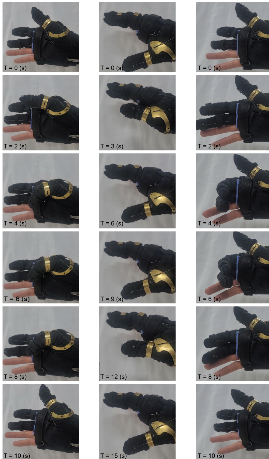
Figure S9: 3 Primitive motions assisted by Exo-Glove Shell
